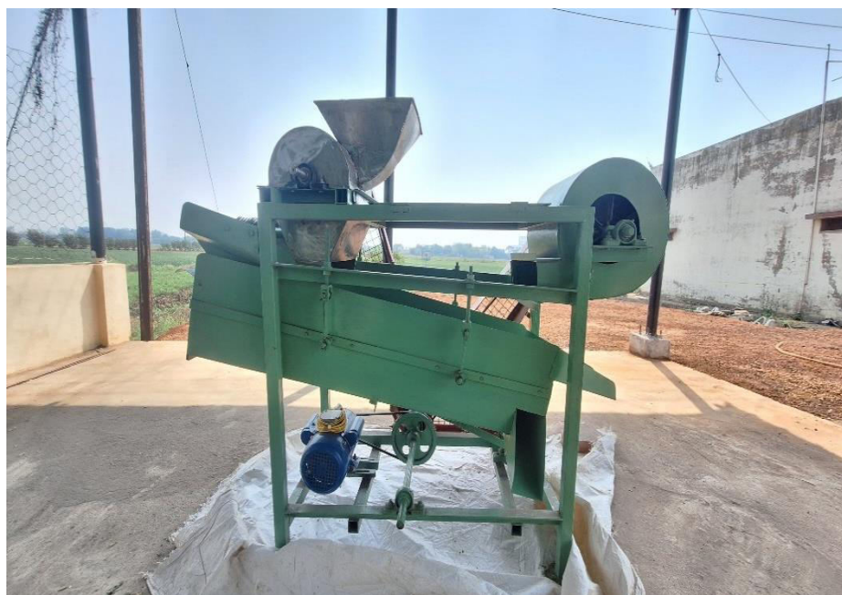
Fig.1 Green chickpea pod stripping cum shelling machine
